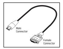
Special Connections Note: Optional DVI to HDMI Adapter Cable For TVs equipped with HDMI, this adapter cable will be required to connect the RJP for digital video/audio.
